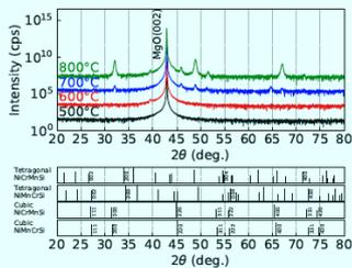
The NiCrMnSi samples were in situ annealed at  $T_a = 500$  and  $700^\circ\text{C}$  before the Ta layer was deposited.
