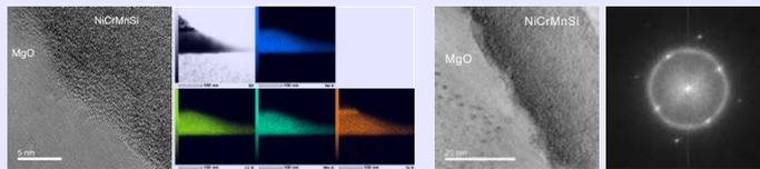
The sample grown at  $T_a = 700^\circ\text{C}$  is epitaxially grown with the grain size of 5~10 nm with interfacial mixing of ~ 20 MLs.
